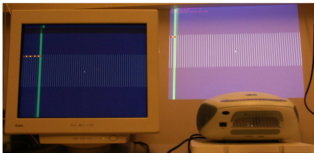
Figure: Comparing the latency of the digital projector with a CRT monitor using the latency tool.
