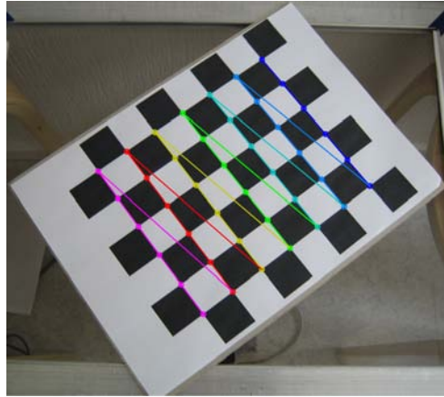
Figure 3.3: Camera image of the chessboard pattern with intersection detected by OpenCV.
