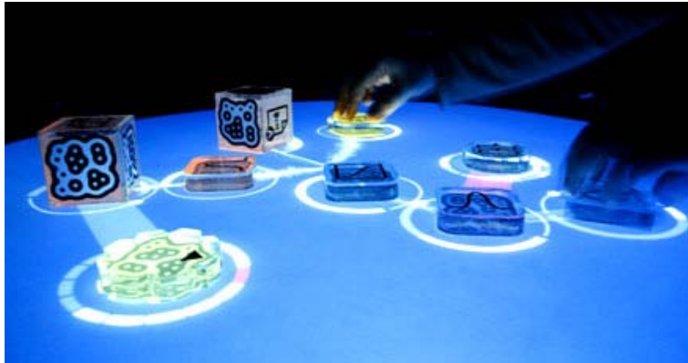
Figure 1.1: Patterns called fiducial markers are attached to physical objects that are recognized and tracked by the reacTable (image taken from [31]).
