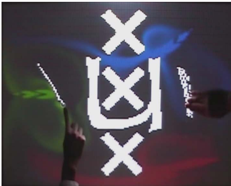
Figure 4.3: Real-time Fluid Dynamics Simulation running in sandbox mode. Two users are drawing boundaries while the simulation is still active.
